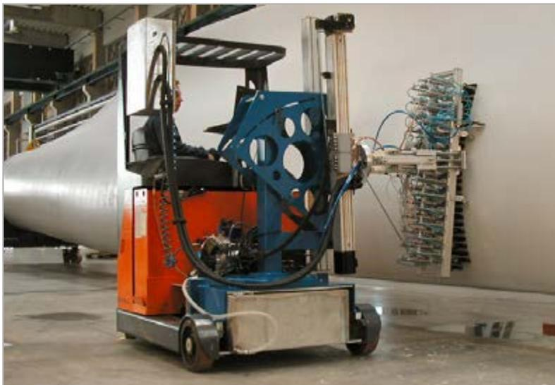
Mobile scanning unit traversing a large turbine blade
