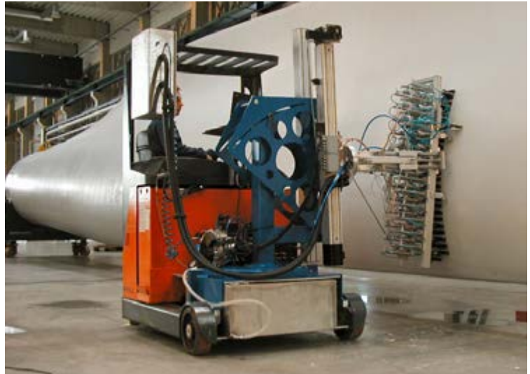
Mobile scanning unit with P-Scan traversing a composite wind turbine blade
