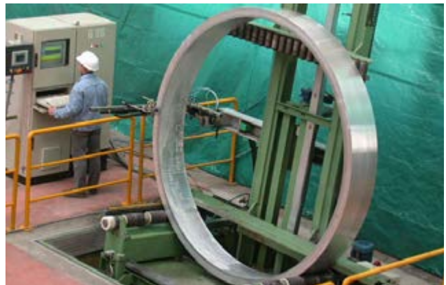
P-Scan 4 ultrasonic scanner and assembly being used to scan a rectangular cross-section forged ring for material homogeneity and defects prior to final machining
