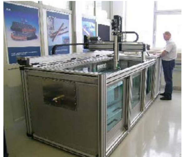
2,400 liter ultrasonic immersion tank
