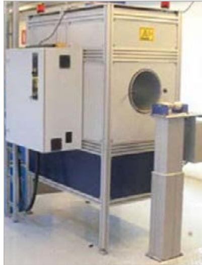
X-ray cabinet system for testing pre-insulated heat pipe systems during production
