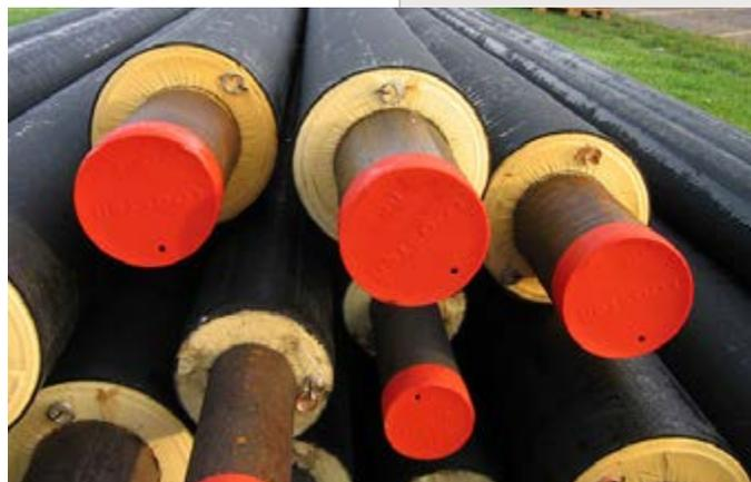
Sections of insulated heat pipe with embedded sensors
