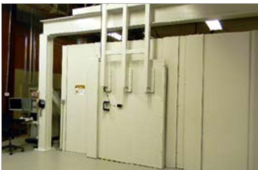
Walk-in custom radiation enclosure for conducting high-energy CT scanning
