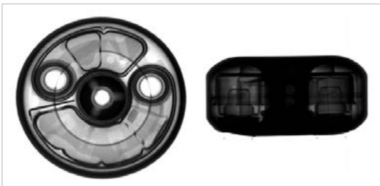
Driver-side airbag containing the igniter system
