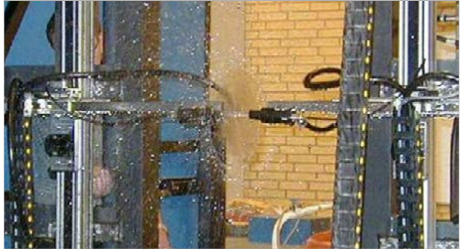
Water jet probe scanner with integrated P-Scan 4 ultrasonic inspection system being used to scan a critical aero structure component
