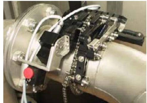
The APS-6 confined-space ultrasonic pipe inspection scanner unit
