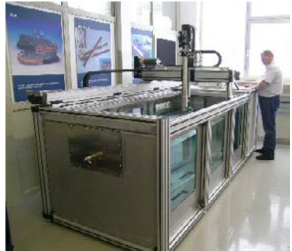
2,400 liter ultrasonic immersion tank
