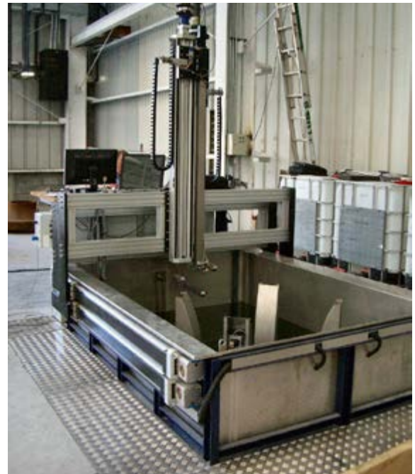
Ultrasonic deep immersion tank for evaluating very large objects
