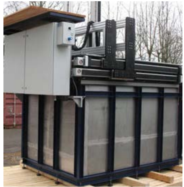
Tank and scanner assembly for inspecting metal forgings, prepared for shipping
