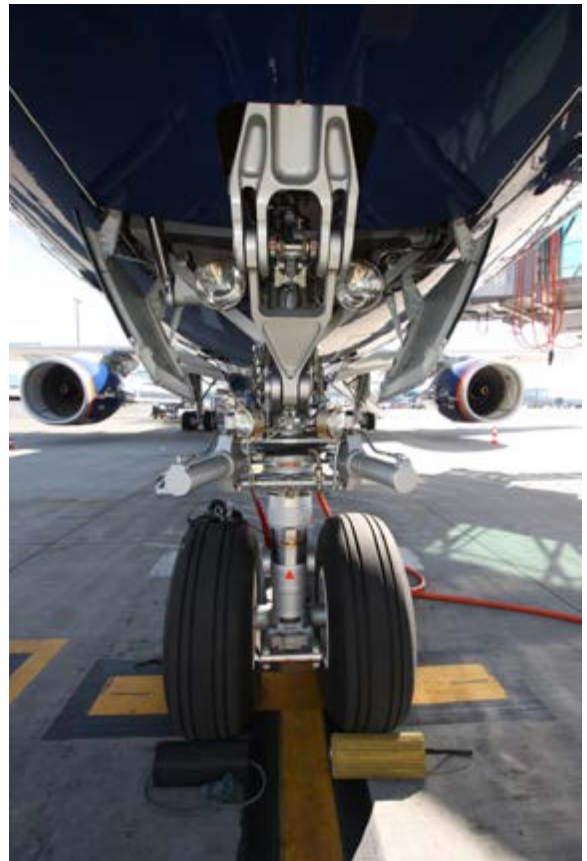
Aircraft landing gear made with high-strength steel components
